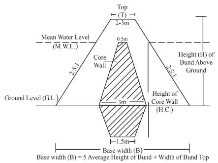
3. Percolation tanks store water for recharging ground water, raising the water table. They are constructed across natural streams and nalas to collect and impound surface runoff water and store it to facilitate infiltration and percolation of water into the sub-strata of the soil, thereby raising the ground water table. Spillways are to be provided for as required.
